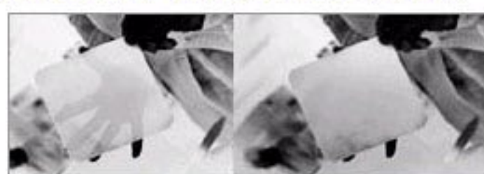
5.5 \mu m band 9.5 \mu m band Dual-band infrared imaging detectors that deliver images in two infrared bands
